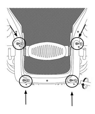
Screw the 4 bolts into the back of the mesh
