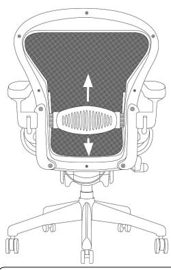
To adjust the lumbar pad - slide it up or down the rails, or switch the pad around to the other side. The pad is double sided one side being firmer than the other
